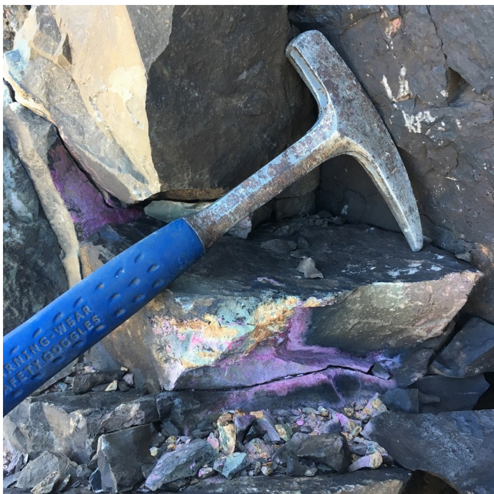
New copper cobalt showing near the Bloom Target at the Monster Property
